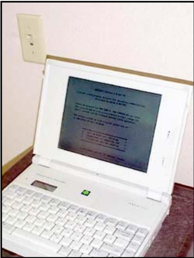
Here's a recycled Zenith 386-class machine with a monochrome display and a 40 MB hard drive. During boot-up it draws 1 A, and in standby it sleeps at about 200 mA. [Photo by KB9EZZ]
