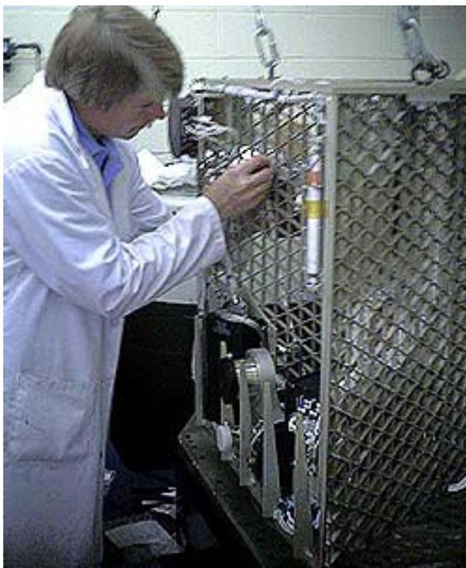
*A University of Alabama-Huntsville engineer attaches part of the PEST electronics to the grid frame that forms the skeleton of JAWSAT. [NASA/Marshall]*
