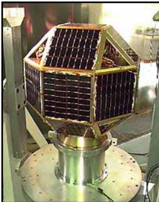
**The PANSAT satellite package after initial integration. [NPS Photo]**
